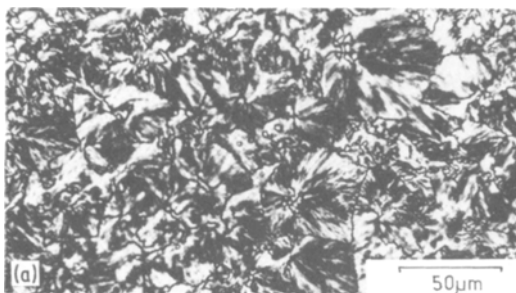
Figure 9 The influence of processing conditions on the morphology of Layer 5. Barrel temperatures: (a) 493 K, (b) 473 K, (c) 453 K.
